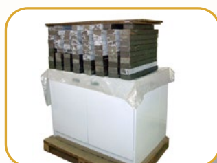
Actual photo during Cabinet Load Testing
