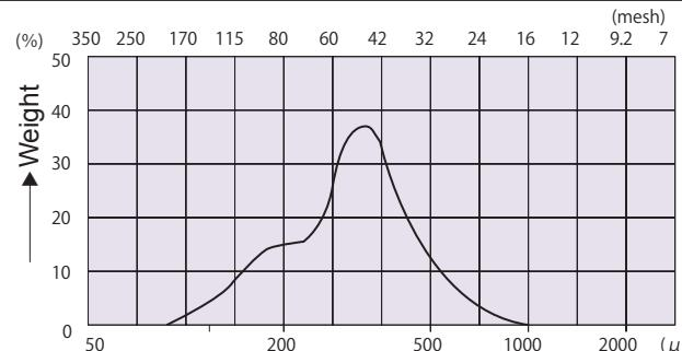
Particles generated by the pulvis mini bed are usually in the range of 0.1~1.5a. The particle size uniformity is lower than extrusion granulation and compression granulation methods.
