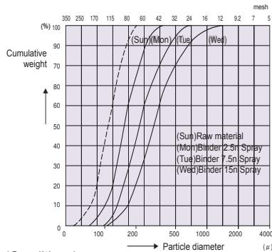
The factors that influence the particle diameter are the binder liquid feed rate and the spray pressure, the former being the most influential. A higher binder amount will result in larger diameter particles.
